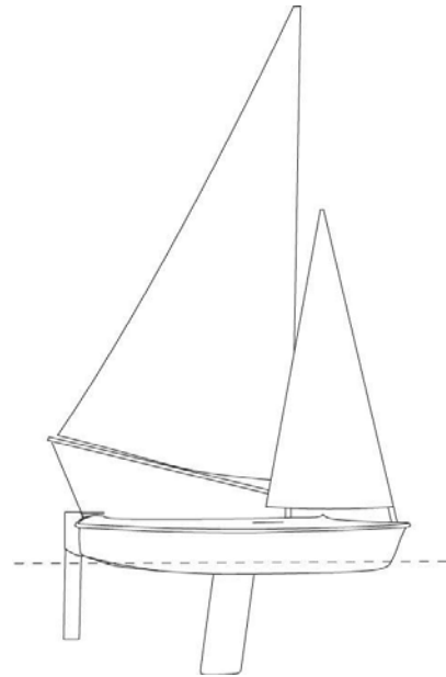
Hansa 303 3m Schooner Rigged Single or Two Person Conventional Jib Single Rudder Blade
