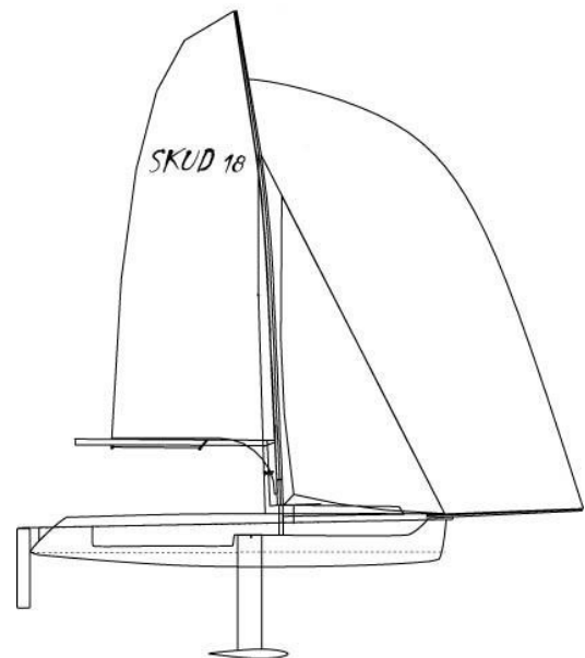
SKUD 18 5.8m Sloop Rigged Two Person Self Tacking Jib Asymmetric Gennaker Twin Rudder Blades
